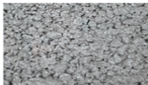
Porous Concrete (PC)
