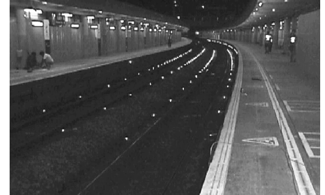
Fig. 3 Prisms mounted on the track sleepers
