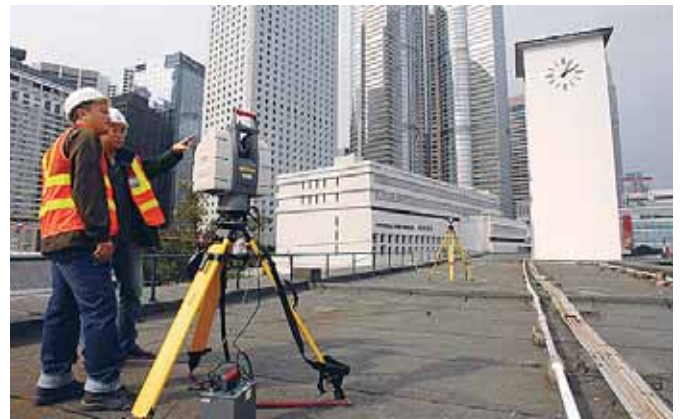
Fig 4 The 3D laser scanning system Leica HDS3000 at the Old Star Ferry Pier
