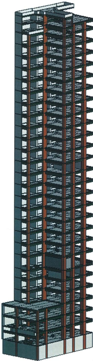
Figure 7 – BIM Structural Model for a Office Building
